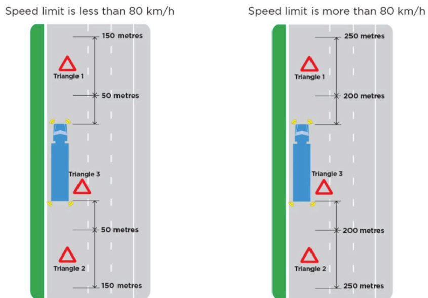
Figure 4.0 Recommended Emergency Triangle Placement
